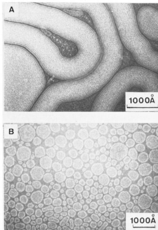
**Figure 4.** Electron micrographs negatively stained with uranyl acetate: A, 5 mM aqueous dispersion of  $CAC_2N^+C_5Sar_2C_{12}$  (magnification,  $\times 132\,000$ ); B, 5 mM aqueous solution of  $CAC_2N^+C_5Sar_2C_{12}$  sonicated for 2 min at a 30-W power level and allowed to stand for 10 min at 5 °C (magnification,  $\times 94\,000$ ).
