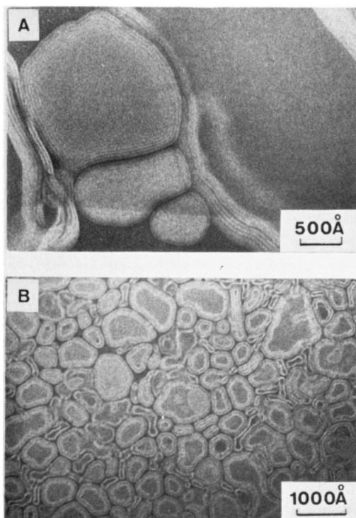
**Figure 7.** Electron micrographs negatively stained with uranyl acetate: A, 5 mM aqueous dispersion of  $N^+C_5Leu_3C_{12}$  (magnification,  $\times 156\,000$ ); B, 5 mM aqueous solution of  $N^+C_5Leu_3C_{12}$  sonicated for 2 min at a 30-W power level and allowed to stand for 10 min at 5 °C (magnification,  $\times 94\,000$ ).
