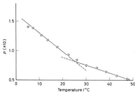
**Figure 2.** Correlation between fluorescence polarization ( $P$ ) of DSTA ( $5.3 \times 10^{-6}$  M) and temperature in single-walled vesicles of  $N^+C_5Leu_2C_{12}$  ( $7.62 \times 10^{-4}$  M) dispersed in aqueous phosphate buffer [pH 6.94 and  $\mu = 0.10$  (KCl)].
