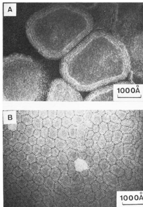
**Figure 5.** Electron micrographs negatively stained with uranyl acetate: A, 5 mM aqueous dispersion of  $N^+C_5Leu_2C_{12}$  (magnification,  $\times 109\,000$ ); B, 5 mM aqueous solution of  $N^+C_5Leu_2C_{12}$  sonicated for 2 min at a 30-W power level and allowed to stand for 10 min at 5 °C (magnification,  $\times 97\,000$ ).
