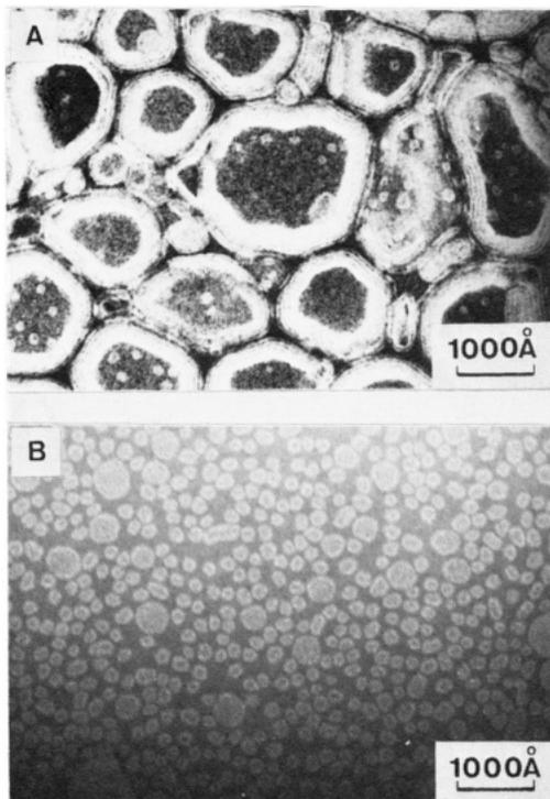
**Figure 3.** Electron micrographs negatively stained with uranyl acetate: A, 5 mM aqueous dispersion of  $N^+C_5Ala_2C_{12}$  (magnification,  $\times 94\,000$ ); B, 5 mM aqueous solution of  $N^+C_5Ala_2C_{12}$  sonicated for 2 min at a 30-W power level and allowed to stand for 10 min at 5 °C (magnification,  $\times 94\,000$ ).
