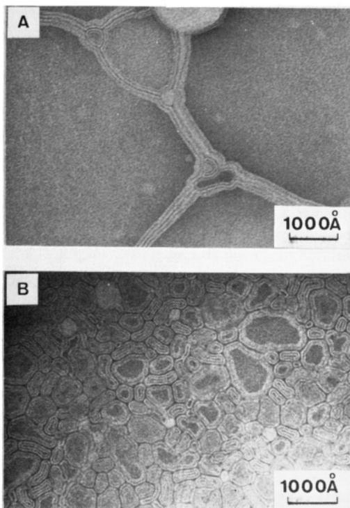
**Figure 6.** Electron micrographs negatively stained with uranyl acetate: A, 5 mM aqueous dispersion of  $CAC_2N^+C_5Leu_2C_{12}$  (magnification,  $\times 94\,000$ ); B, 5 mM aqueous solution of  $CAC_2N^+C_5Leu_2C_{12}$  sonicated for 2 min at a 30-W power level and allowed to stand for 10 min at 5 °C (magnification,  $\times 94\,000$ ).
